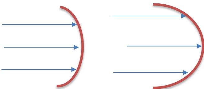
3. Adjust the angle of the mirrors so that all the rays pass through one point (the FOCUS)
