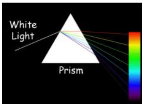
The optical system which allows production and viewing of the spectrum is called a spectroscope.
